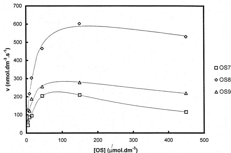
**Figure 4.** Function of  $v = f([\text{OS}])$  at the lowest concentration of XG used ( $67 \text{ mg} \cdot \text{dm}^{-3}$ ) showing the inhibition of the reaction at high concentrations of OS. Data were fitted to the rate equation for a single substrate reaction exhibiting substrate inhibition.
