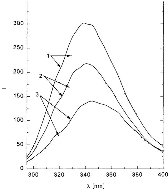
**Figure 5.** Fluorescence emission spectra of  $\alpha_1$ -AG(-Sia,-1 comp) at different temperatures. Increasing temperature (1) — 25°C, (2) — 50°C, (3) — 75°C. Decreasing temperature (1) 25°C, (2) 50°C, (3) 75°C.
