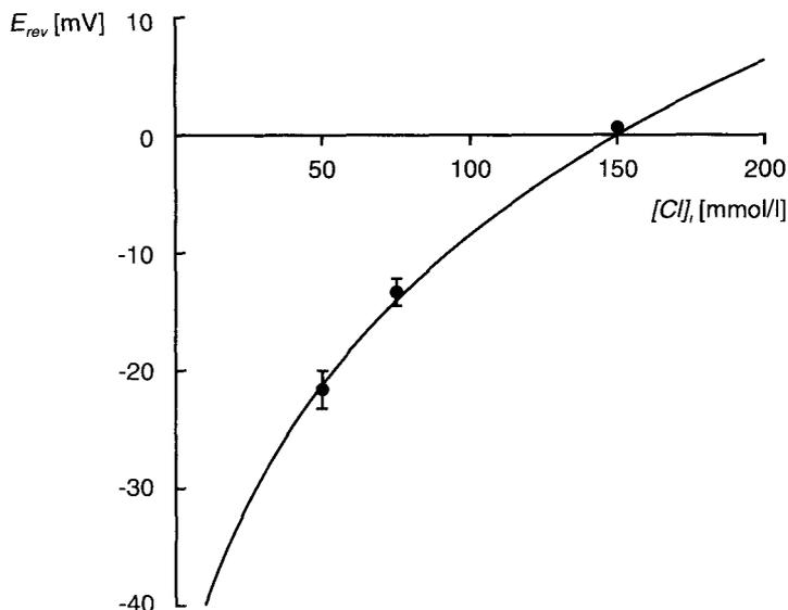
**Figure 3.** The dependence of the reversal potential,  $E_{rev}$  on the internal concentration of chloride ions,  $[Cl]_i$ . The curve was fitted according to Eq. 1 with  $P_{Na}/P_{Cl} = 0.15$ .
