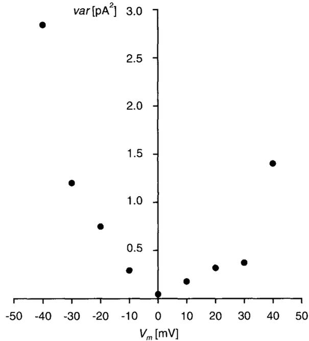
**Figure 2.** Variance,  $\text{var}(pA^2)$  of the open state currents at different membrane potentials,  $V_m$  (from  $-40$  to  $+40$  mV at 10 mV steps) as measured in the absence of closed states. For explanation see text (Symmetrical 145 NaCl, 0.5 CaCl<sub>2</sub> solutions (in mmol/l)).
