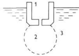
**Fig. 1.** A schematic outline of the system used to study volume flow in spherical membranes. 1, 2 and 3 are solution compartments separated by the capillary and the membrane. We assume that compartments 1 and 3 are large and stable as compared to compartment 2.
