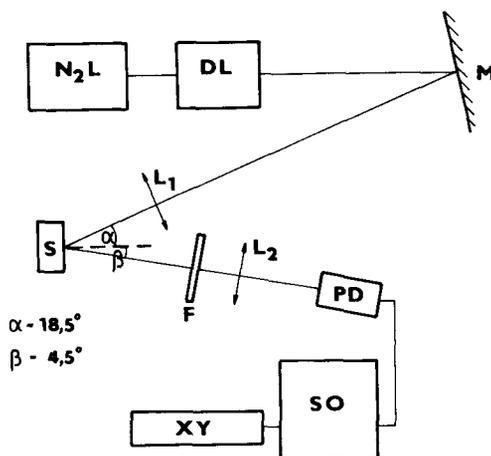
**Fig. 1.** Scheme of the optical and electrical set-up ( $N_2L$  — nitrogen laser, DL — dye-laser, M — mirror, S — sample, F — optical filter,  $L_1, L_2$  — lenses, PD — PIN diode, SO — Sampling Oscilloscope, XY — recorder).
