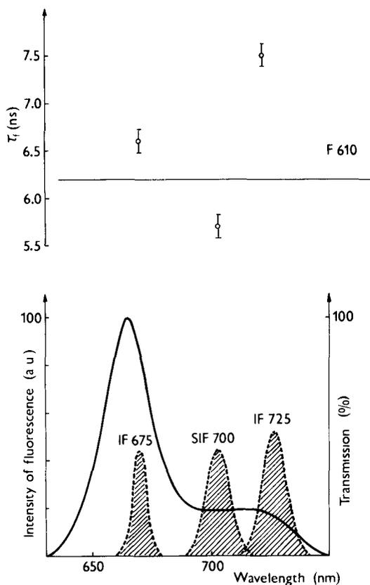
**Fig. 2.** Fluorescence spectrum of Chl *a* in n-hexane ( $C = 7.6 \times 10^{-5} \text{ mol} \cdot \text{l}^{-1}$ ), transmission curves of interference filters, and the corresponding  $\tau_f$  values.
